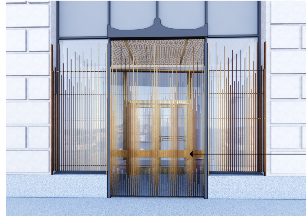
EMERGENCY DOOR HARDWARE
